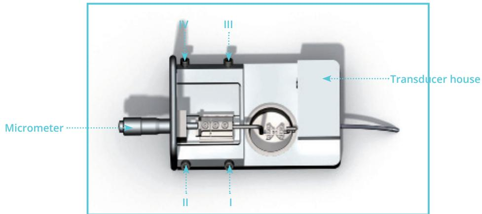
Figure 4.2 Fine adjustments of the jaws in the myograph chamber
