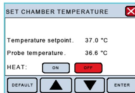
To turn the heat on, touch “ON” and the “ON” icon will turn green, indicating the heat has been turned on. The system will heat to the designated temperature setpoint.
