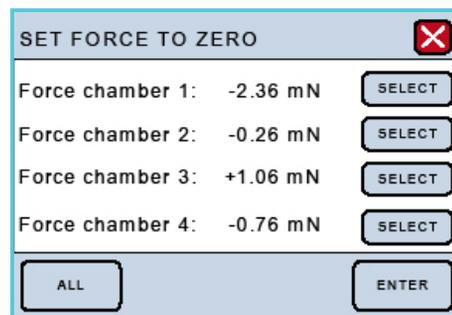
The line to be modified will turn blue, indicating that the interface is waiting for input. When "ALL" is chosen, all lines corresponding to all 4 channels will turn blue. Changing the numeric value for the chosen parameter can be done by touching the up or down arrow keys.
