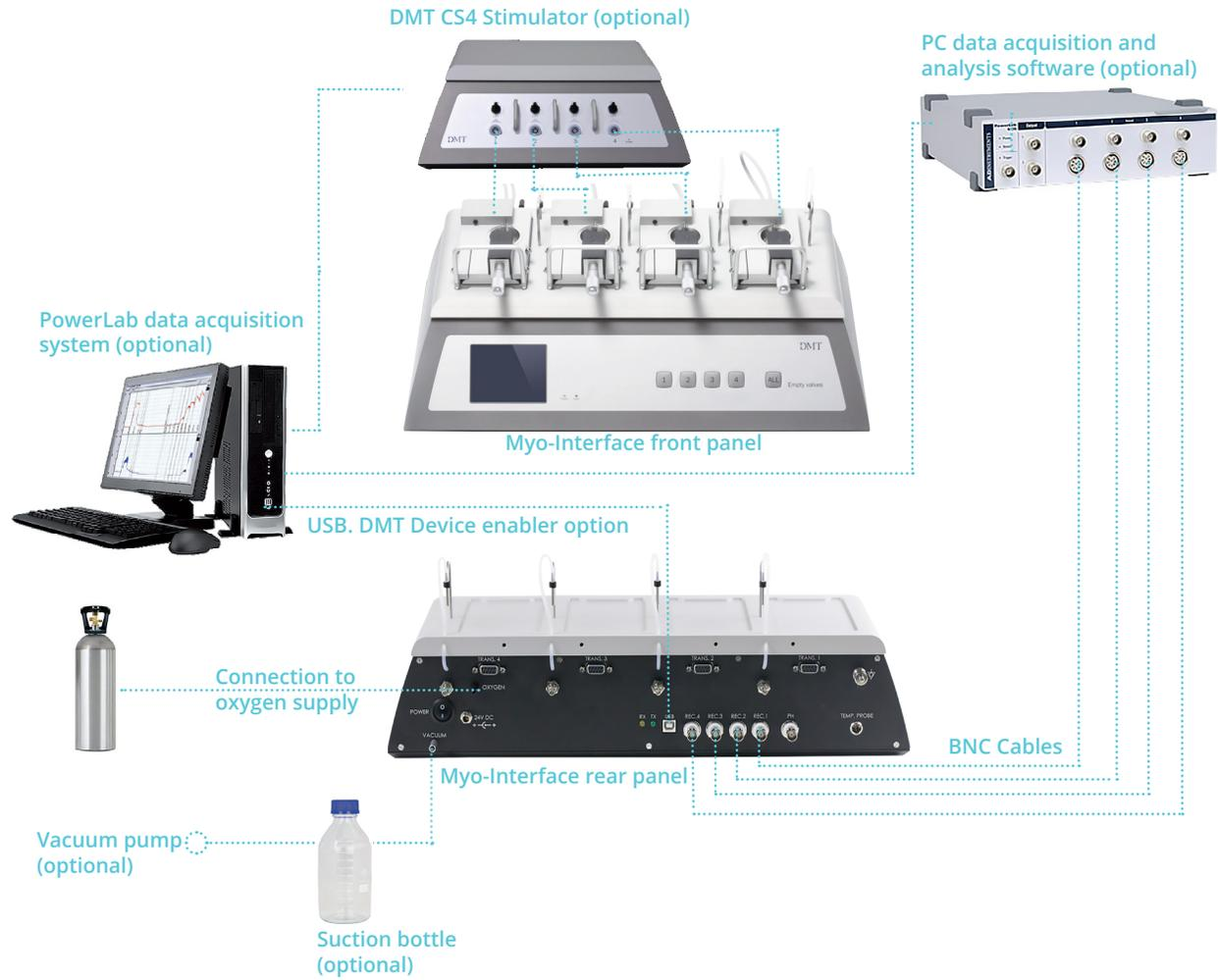
Figure 2.1 The complete Multi Wire Myograph System - Model 620M
