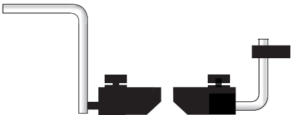
Figure 1.5 Mounting jaws for small vessels - Side View
