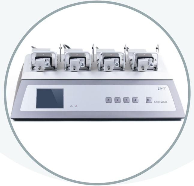
Making it easier... the newly developed 4-channel system adds the ease of automating the normalization procedures so that calculations and preload tension is easily set. Following mounting and equilibration, passive length-tension relationships are determined by a standardized procedure. This allows the standardization of initial experimental conditions, an important consideration when examining pharmacological differences between vessels.
