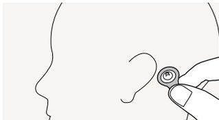
3 Place the second electrode (DRL) inferiorly to the CMS electrode.
